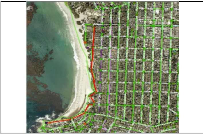
Photo: Pipe Bursting Limits on Scenic
