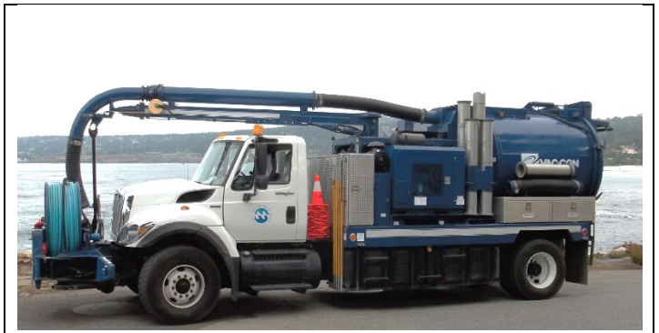
Photo: CAWD Vactor Truck
